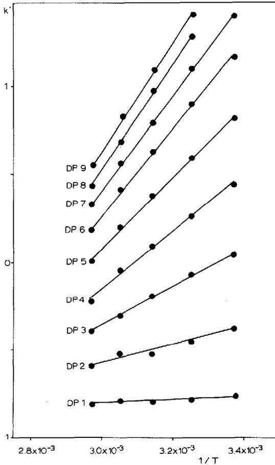
Fig. 7. Van 't Hoff lines for maltodextrin series. Chromatographic conditions and designation of saccharides as for Fig. 3.
