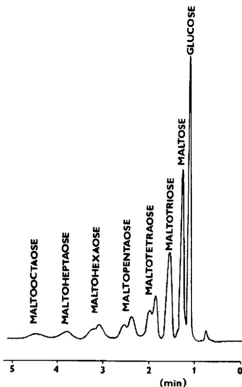
Fig. 2. Separation of maltodextrins by reversed-phase liquid chromatography. Glass cartridge, 150 × 3.2 mm. Sorbent: silica C<sub>18</sub> 5  $\mu\text{m}$ . Eluent: water. Flow-rate: 54.1 ml/h. Column temperature: 24°C. Pressure drop: 15 MPa. Sample introduction: stop-flow valve. Detector: refractometer.
